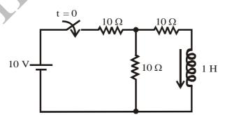
The value of V that would result in a steady-state current of 1 A through the inductor in the above circuit is
