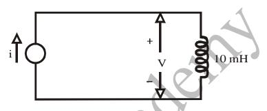
In the above shown circuit, the independent current source generates zero current for t < 0 and a pulse 5 t  $e^{-4t}$  A, for t > 0. At what instant of time, will the current attain the maximum value in the circuit?
