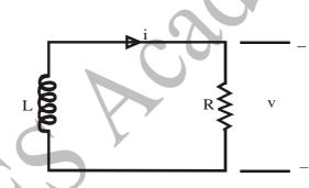
Voltage and current expressions for the above circuit are given at  $t \ge 0$  as v = 125 $e^{-50t}$  V,  $i = 5 e^{-50t}$ A. The value of L will be
