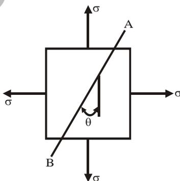
A point in two-dimensional stress state, is subjected to biaxial stress as shown in the above figure. The shear stress acting on the plane AB is
