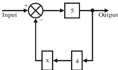
The above figure shows the block diagram of an automatic control system having bounded input. The output becomes unbounded if the value of  $x$  is
